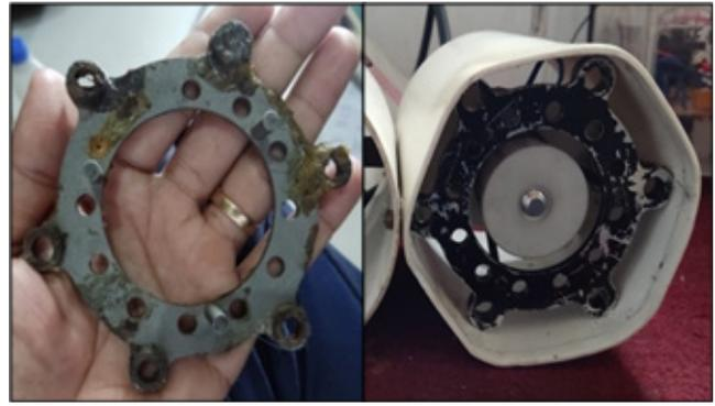
Gambar 14. Reflector Transmitter Transducer
