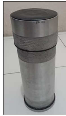
Gambar 9. Transmitter (Tx) USBL.
