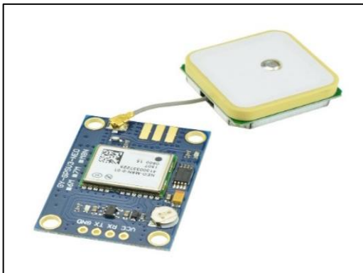
Gambar 2. 4. GPS UBlox Neo-6M 12,2 x 16 x 2,4 mm ( https://www.electroschematics.com/neo-6m-gps-module/ )
