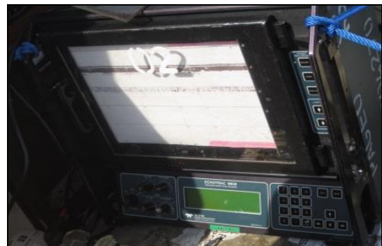
Gambar Singlebeam Echosounder (Echotrac MK III)
