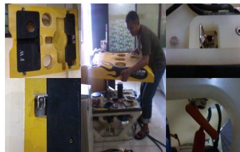
Melepas main buoyancy block
