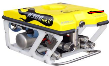
Memasang main buoyancy block
